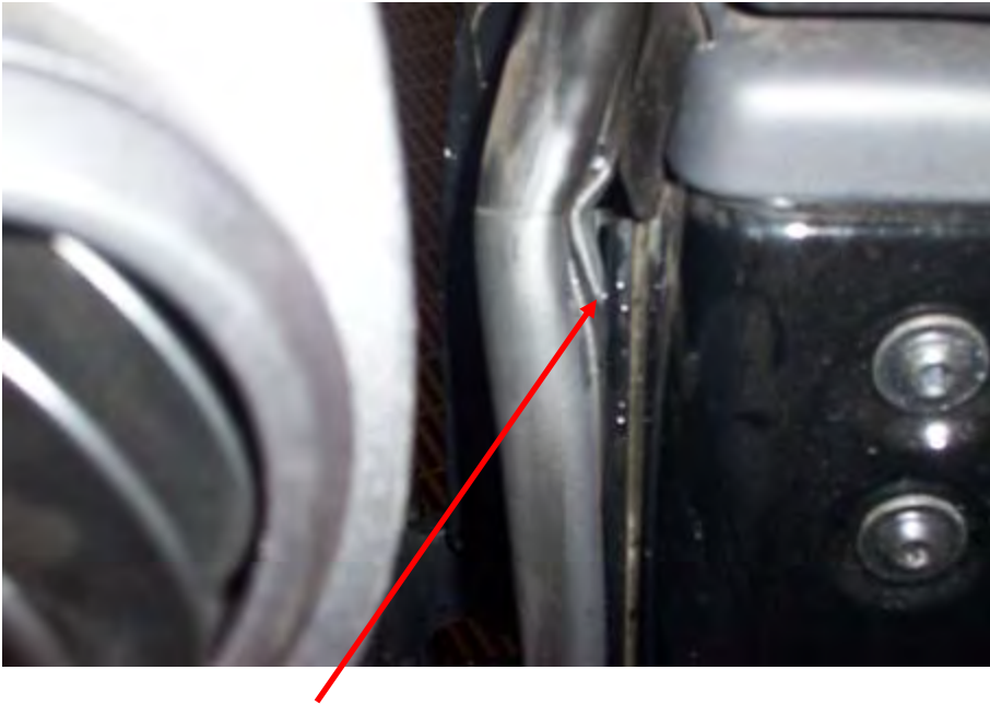
Seal is not seated in channel
