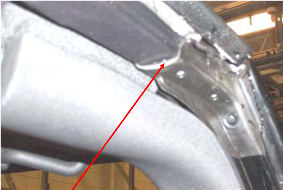
Header Seal Cup Folded under
